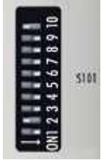
Fig. 18: DIP switch S001: Left off "0", right on "1"
