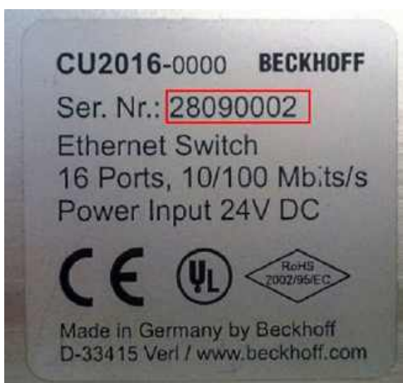
Fig. 3: CU2016 switch with serial/ batch number
