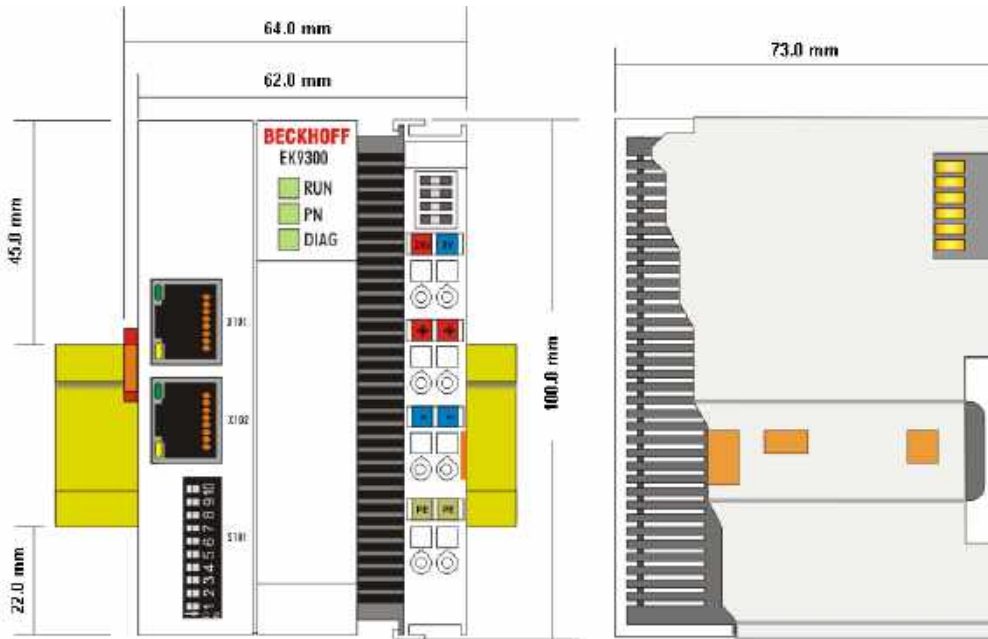
Fig. 11: EK9xxx – dimensions taking the EK9300 as an example
