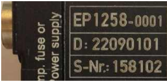
Fig. 5: EP1258-0001 IP67 EtherCAT Box with batch number/ date code 22090101 and unique serial number 158102
