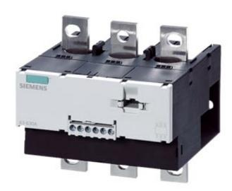
CURRENT/VOLTAGE MEASUR. MODULE; SET CURRENT 63...630A; VOLTAGE DETECTION UP TO 690V; OVERALL WIDTH 145MM; BUS BAR CONNECTION
