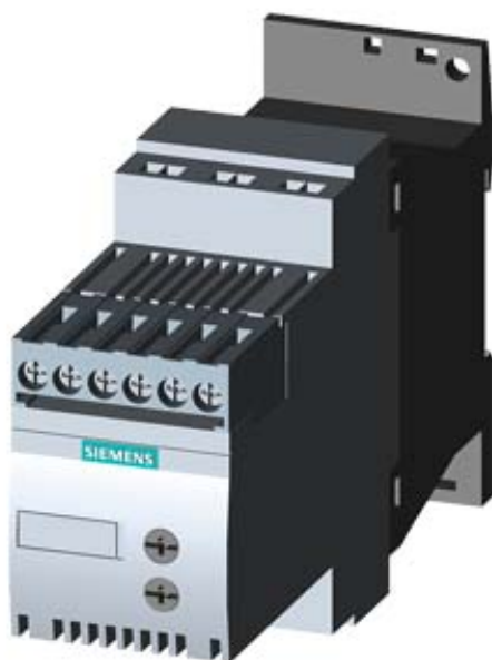
SIRIUS SOFT STARTER, SIZE S00, 17.6A, 7.5KW/400V, 40 DEGREES, 200-480V AC, 24V AC/DC, SCREW TERMINALS
