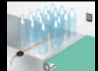
Detecting improperly placed PET bottles
