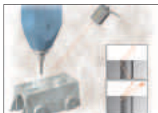
Detecting threading on metal parts
