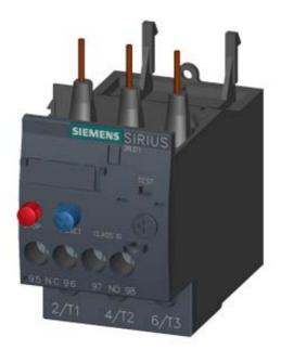
OVERLOAD RELAY 20...25 A FOR MOTOR PROTECTION SZ S0, CLASS 10, F. MOUNTING ONTO CONTACTOR MAIN CIRCUIT: SCREW TERMINAL AUX. CIRCUIT: SCREW TERMINAL MANUAL-AUTOMATIC-RESET
