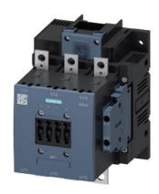
Power contactor, AC-3 115 A, 55 kW / 400 V AC (50-60 Hz) / DC operation 220-240 V UC Auxiliary contacts 2 NO + 2 NC 3-pole, Size S6 Busbar connections Drive: conventional screw terminal
