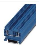
Feed-through terminal block, Connection method: Spring-cage connection, Cross section: 0.08 mm² - 4 mm², AWG: 28 - 12, Width: 5.2 mm, Color: blue, Mounting type: NS 35/7,5, NS 35/15
