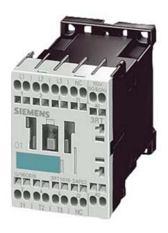
CONTACTOR, AC-3 4 KW/400 V, 1 NC, DC 24 V, 3-POLE, SIZE S00, CAGE CLAMP
