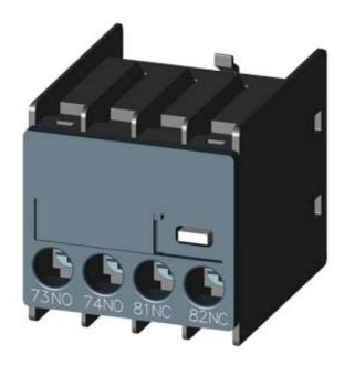
AUX.SWITCH BLOCK,FRONT,1NO+1NC, CURR.PATH:1NO, 1NC, CONN.F.BE., F. CONT. RELAYS A. MOTOR CONT., SZ S00 AND S0, SCREW TERMINAL 73 / 74, 81 / 82
