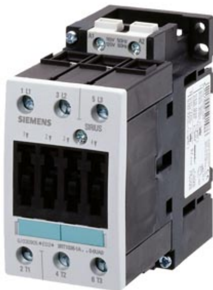
CONTACTOR, AC-3 22 KW/400 V, DC 24 V, 3-POLE, SIZE S2, SCREW CONNECTION
