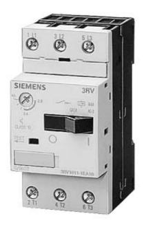
CIRCUIT-BREAKER SIZE S00, FOR MOTOR PROTECTION, CLASS 10, A-REL. 3.5...5A, N-REL. 65A, SCREW TERMINAL, STANDARD SWITCHING CAPACITY
