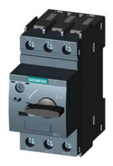
CIRCUIT-BREAKER SZ S0, FOR MOTOR PROTECTION, CLASS 10, A-REL.1.1...1.6A, N-REL.21A SCREW CONNECTION, STANDARD SW. CAPACITY
