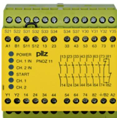
Safety relay (standalone) Inputs: 1- / 2-channel wiring with detection of shorts across contacts Outputs: 7 N/O, 1 N/C, 2 semiconductor. Automatic/monitored start UB 230 - 240 V AC/24 V DC, width: 90 mm, plug-in terminals of screw type Monitoring E-STOP, safety gates.
