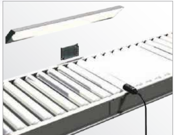
Pulse synchronisation for high ambient light immunity.
